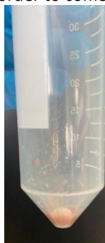
Figure 2. Remove the supernatant, insert the device, wait 10 minutes for absorption of cellular material into the disc
