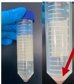
Figure 1. Within a falcon it is necessary to separate the cytological pellet from the supernatant by centrifugation
